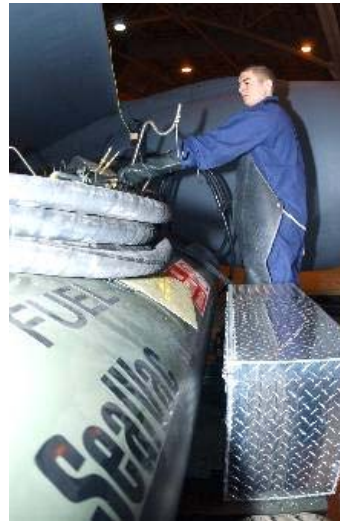
FAIRCHILD AIR FORCE BASE, Wash. -- Senior Airman Nicholas Hamstra applies vacuum pressure to drain fuel from a KC-135 Stratotanker. The fuel bowser allows multiple tanks to be drained safer and quicker than the old draining method. Airman Hamstra is a fuel systems journeyman with the 92nd Maintenance Squadron here. (U.S. Air Force photo by Airman 1st Class Clay Lancaster)
